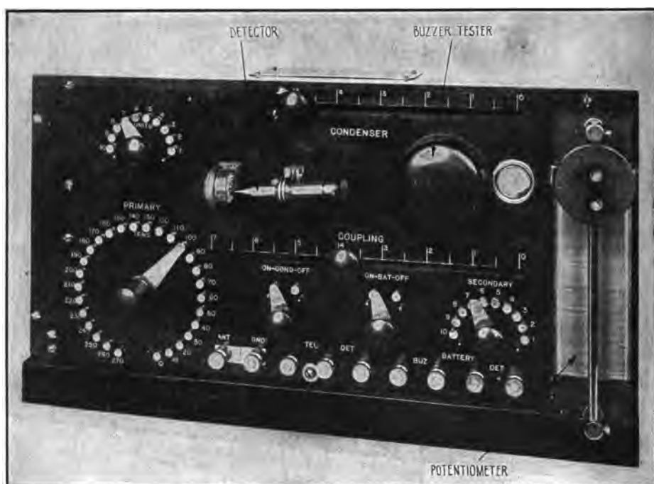
Fig. 203a—Front View of the Marconi Type 112 Receiving Tuner (The American Marconi Company).
